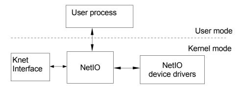
As can be seen, NetIO is a Linux kernel module that interacts with a user process, so that the packet processing is actually performed in user space rather than kernel mode. NetIO device drivers are used to provide the physical device interface.
