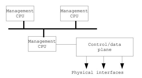
Internally, there are a number of different CPUs, some with functions related to the management facilities of the device (providing user interface, CLI services, configuration, monitoring etc.), and some dedicated to packet processing and control plane functions (route protocol processing etc.).
